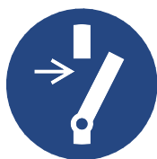
66947 – Inspection cover/inspection door: “Disconnect completely before working”, “Warning of risk of crushing”
