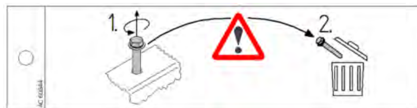
60844 - Transport safety screw (with hydroBLU)
