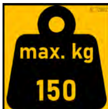
72882 – Maximum permissible load on the unit surface
