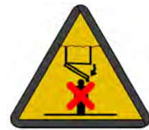
66945 – Warning “Do not stand within the units' swivel ranges”
