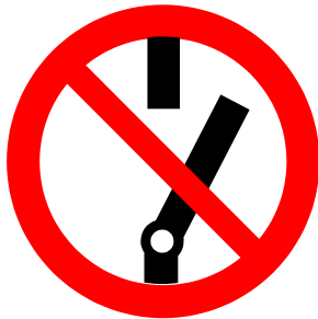
Fig. 2: Example for a warning sign when securing the machine against being switched on again
