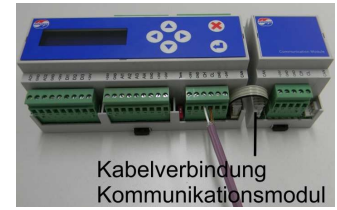
Cable Connection Commu- nication Module
