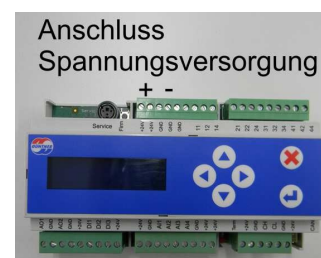
Power supply connection + -
