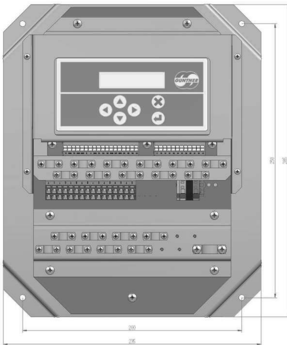
Fig. 12.3: GMM EC/01 /04 /08 UL housing dimensions
