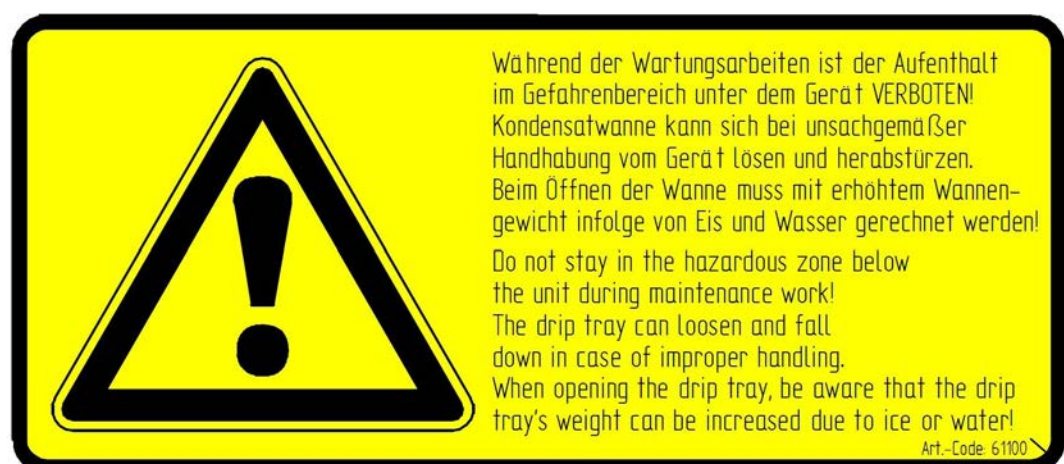
61100 - Tray safety catch warning sign
