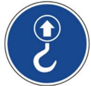
Label 3: 64620 – Lifting point
