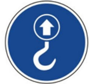
Label 3: 64620 – Lifting point
