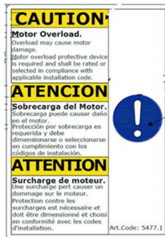
Label 14: 5477.1 - Caution of motor overload
