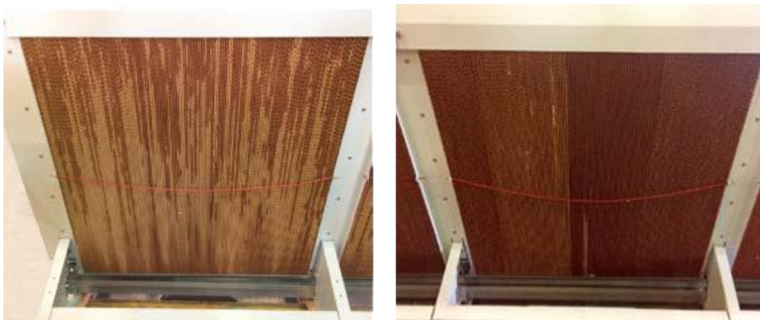
Figure 4. Water distributes from above the media pads, which transition from dry to saturated.
