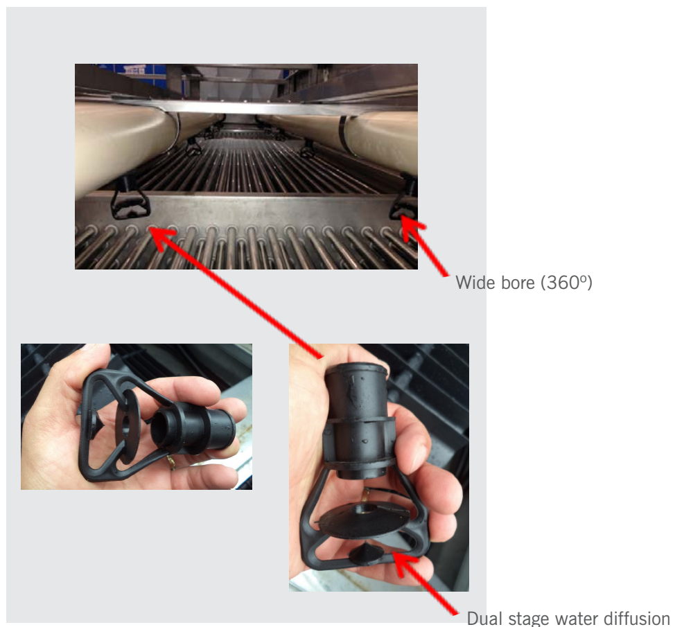
Figura 7: Position and distribution of water from the nozzle
